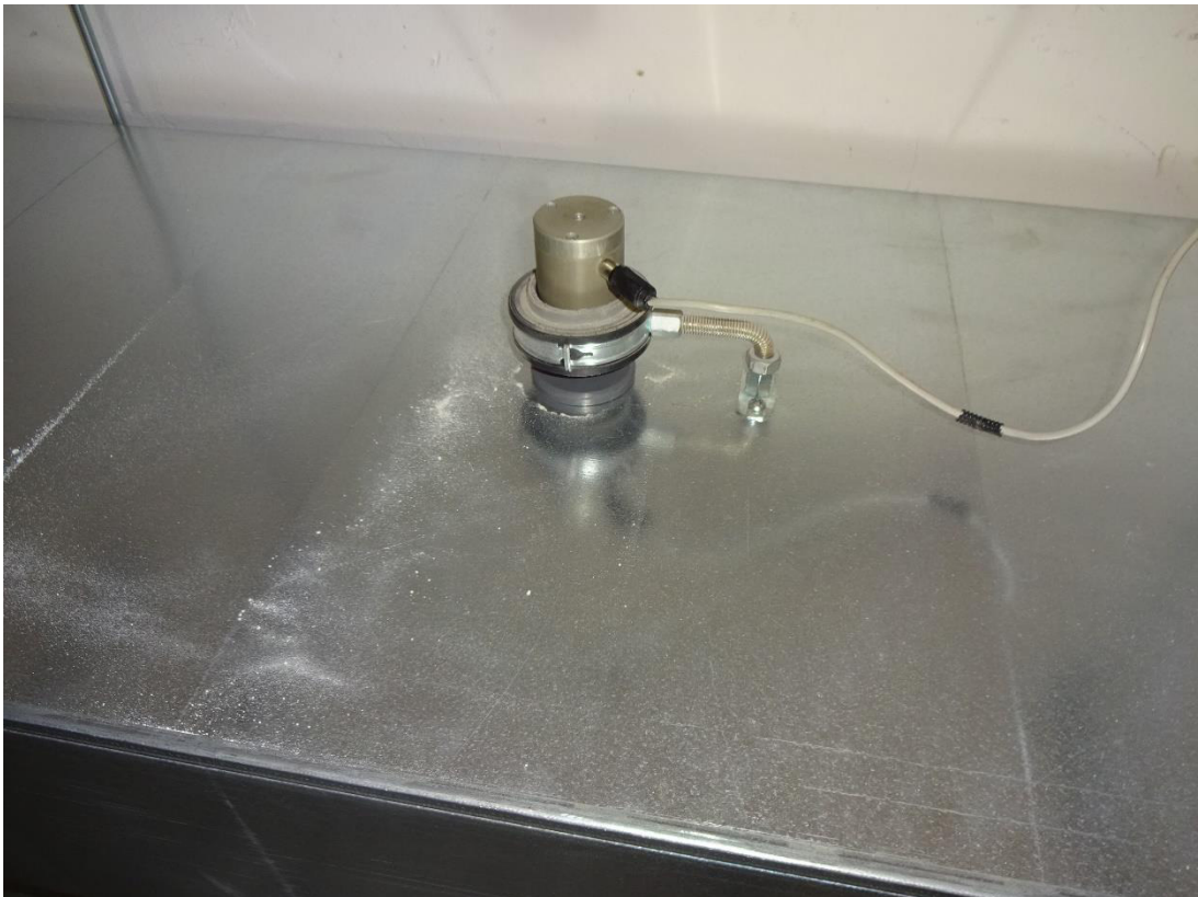
Fig. 2: Reference: ventilation duct, placed on MPC system rails (38/40/2.0) without DÄMMGULAST® rail profiles
